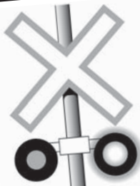
crossbuck with flashing red lights
